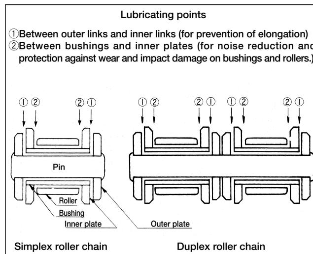
Lubricate on the sag side of the chain, i.e., at the position indicated in the following illustration. Since the lubricant is also useful for rust prevention, coating the entire surface of the chain with the oil is recommended.
